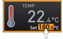
3. Save the set value by pressing the confirmation key. The display returns to normal and the appliance begins adjusting to the defined set value.
