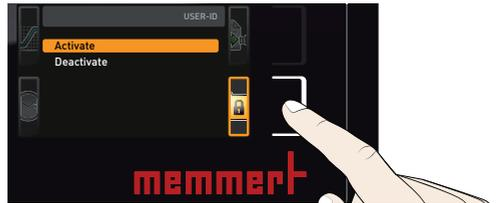
3. Confirm the activation by pressing the confirmation key. The new user ID data are transferred from the USB storage medium and activated. As soon as activation is complete, a check mark appears in front of the corresponding entry.
