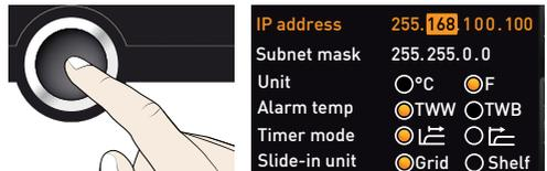
5. After setting the last three digits, accept the new IP address by pressing the confirmation key. The selection returns to the overview.
