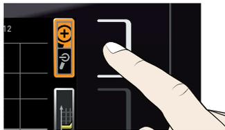
To close the graphical representation, again press the activation key which you have used to activate it.
