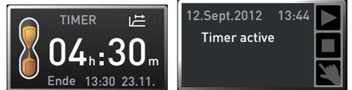
4. Now, as described under 5.4.2, set the individual values for temperature, air flap position etc. which you want the appliance to operate at. It is not possible to change any parameters while the timer is counting down.
