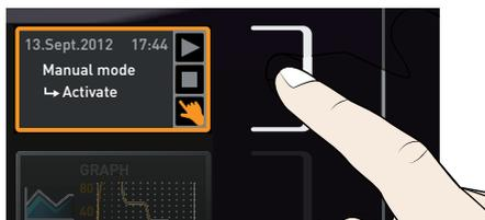
2. Turn the turn control until the ▶ start symbol is highlighted. The current programme is displayed, in this example Test 012.
