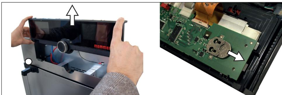
Fig. 30 Removing the lithium battery
