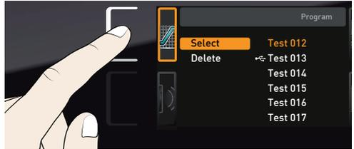
2. Call the Select function by pressing the confirmation key. All programmes available are displayed, including the ones saved on the USB storage medium (identified by the USB symbol). The programme currently available for use is highlighted in orange.
