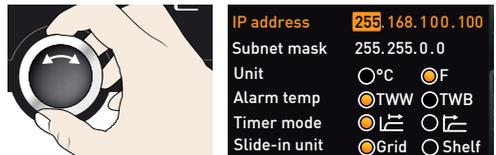
4. Accept the selection by pressing the confirmation key. The next three digits of the IP address are automatically selected. Setting these is done according to the description above.
