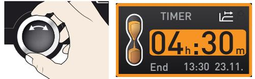
**i** Up to a duration of 23 hours 59 minutes, the time is displayed in hh:mm (hours:minutes) format. For 24 hours and more, the format dd:hh (days:hours) is used. The maximum duration adjustable is 99 days 00 hours.
