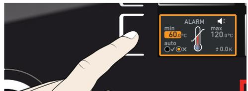
2. By turning the turn control, adjust the desired lower alarm limit value, in the example on the right 160 °C.
