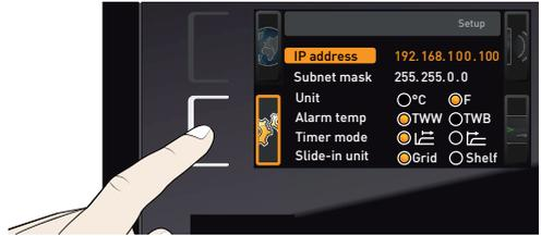
2. Accept the selection by pressing the confirmation key. The first three digits of the IP address are automatically selected.
