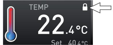
Fig. 29 Temperature adjustment at appliance locked (example)
